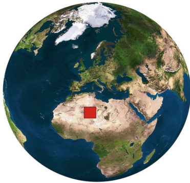
Figure 2: Area of land that needs to be covered with 10% efficient solar cells in order to generate 20 TW of electrical power. 4
