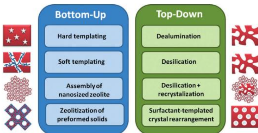
Figure 8: Classification of the techniques to obtain hierarchical zeolites, categorised into the two main "bottom-up" and "top-down" approaches. 42
