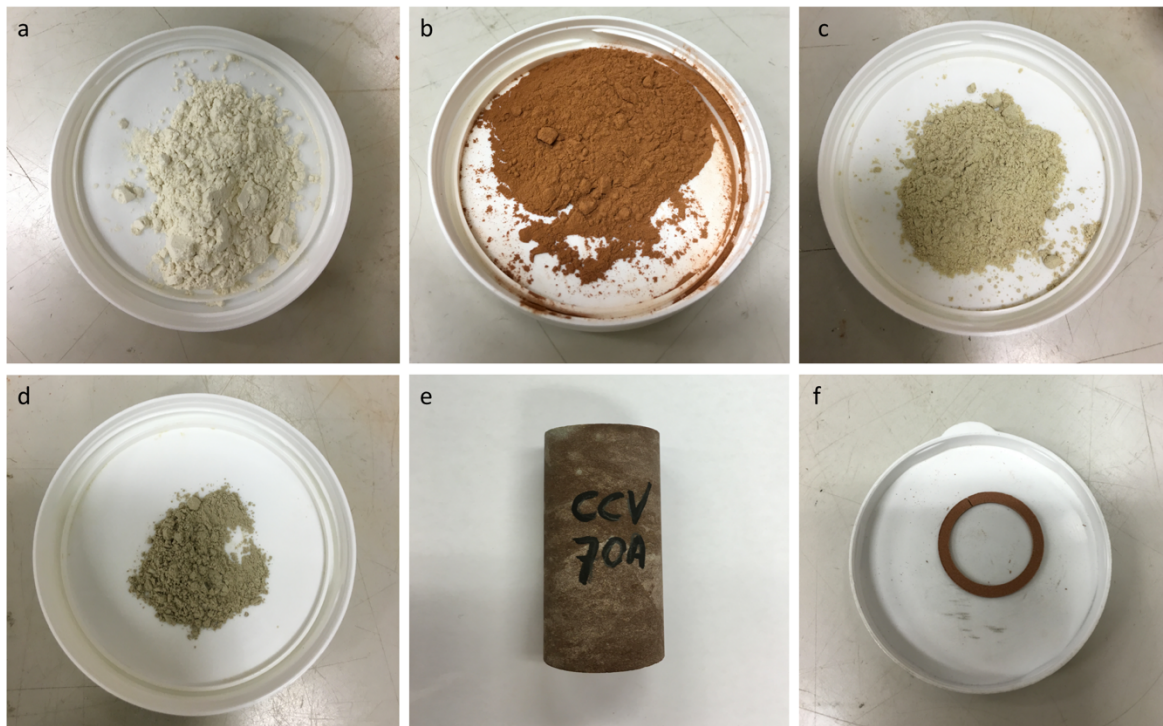
Figure 3: Sample material used in this study in powder form. (a) white illite clay, (b) red illite clay, (c) green illite clay, (d) red illite clay processed with sodium dithionite (hematite is dissolved), (e) Carmel CCV-70A sample, (f) ring shaped pressed sample with an inner diameter of 22 mm, an outer diameter of 28 mm and thickness of ~1 mm.
