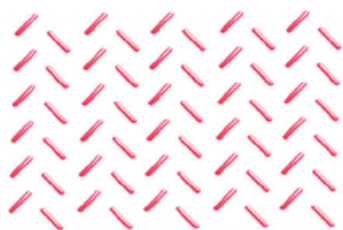
2.4 (A) The Herringbone packing causes inferior carrier mobility.
