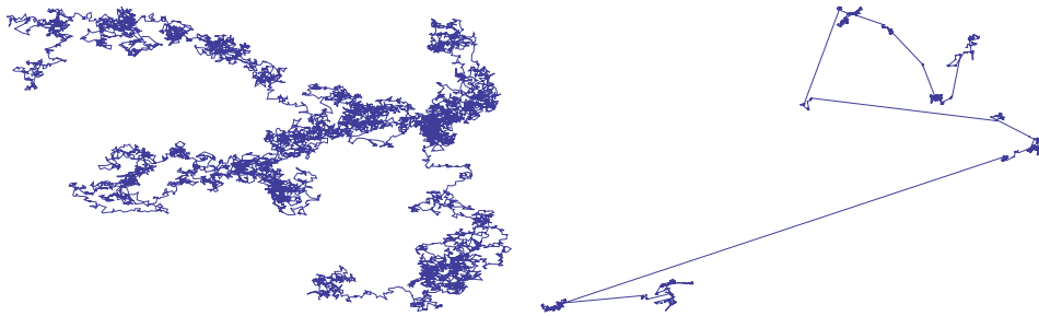
Figure 1.4 – Two-dimensional random walks based on Brownian motion (left) and the Cauchy process (right). The length scales can be set by the parameters of the distributions, so they are arbitrary and therefore not shown in the figures. The discontinuous jumps of the Cauchy process are clearly not present in the continuous Brownian motion. Note that the random walks consist of the same number of steps.
