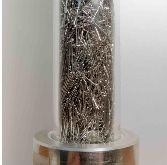
**Figure 3.1:** Separation matrix in a magnetic separation setup. The matrix is composed by ferromagnetic rods made of AluChrom O® from ThyssenKrupp VDM
