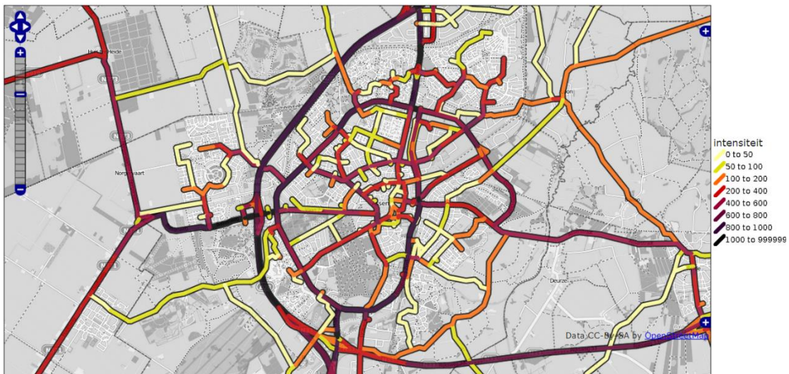
Image 4: Traffic intensity map of the city Assen, created by using the data collected by Dat.Mobility 7 through the Sensor City project. The scale on the right shows the colors that match the intensity levels. 8
