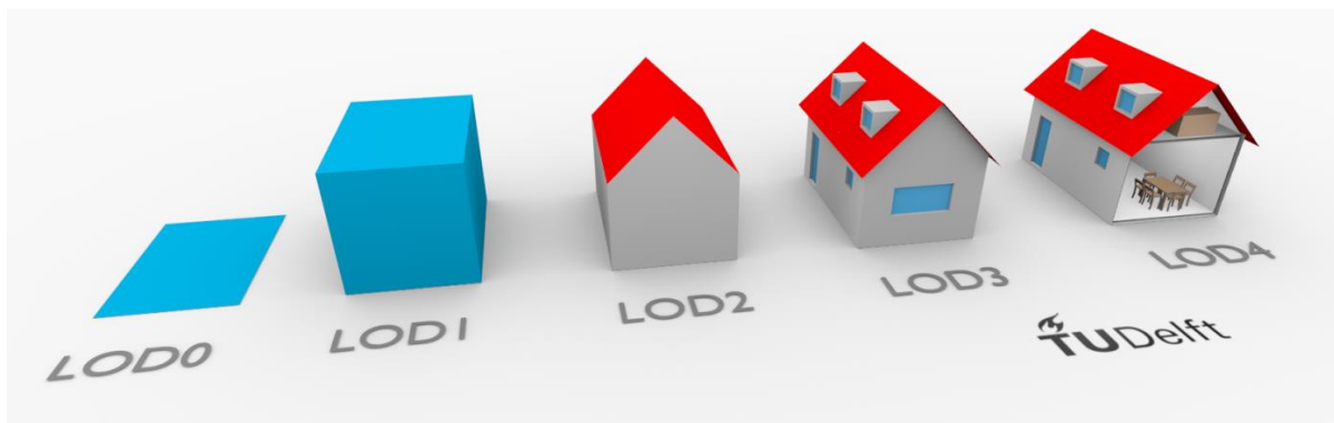
Figure 1: Different Levels of Detail (LoD) according to CityGML; from 2D to 3D (TUDelft, 2015).
