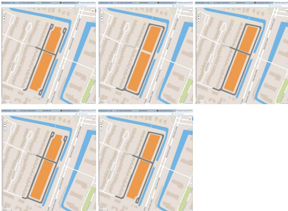
Figure 13: The GeoJSON files of the planning designs, applied in the online PPGIS environment for the NNO project. The GeoJSON objects depicted in orange represent building area, and depicted in grey represent the traffic access scenario's.
