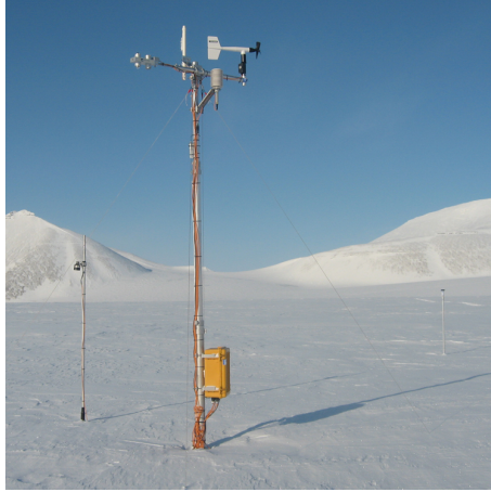
Figure 5: A Sonic height sensor unit placed on Nordenskildbreen left of the Automatic weather station
