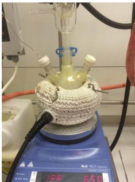
Figure 3.3: Visible vapour formation during the colloidal synthesis.
