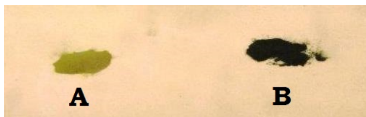
Figure 3.23 Copper(I) acetate (CuOAc) from different bottles of the same supplier. a Light green, from ‘old’ bottle. b Forest green, from ‘new’ bottle. According to the reported synthesis procedure of Yin et al. [37] a forest green CuOAc reagent has to be used.
