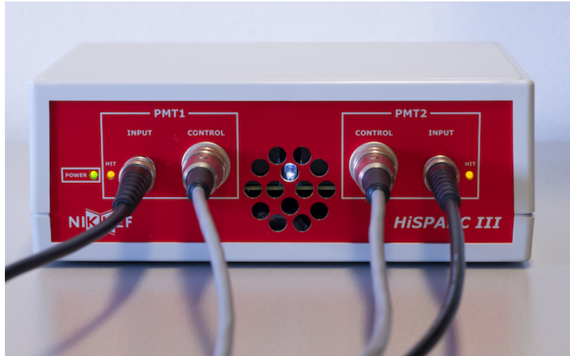
Figure 2.5 – The HiSPARC ‘Red box’ in which the trigger and ADC are located. Two detectors are connected. The blue LED, located in the middle, is turned on, indicating that an event is observed. Image from [de Laet and van Eijk, 2016].
