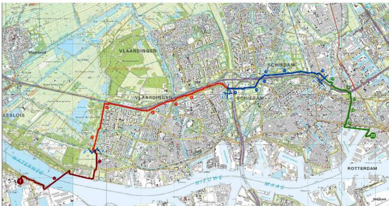
Figure 24 Map showing the route of Leiding over Noord. Point 1 marks the AVR waste incineration plant. Point 20 marks heat station Galileistraat, the former CHP plant now converted to transfer heat with the existing district heating network. From: Eneco (n.d.).
