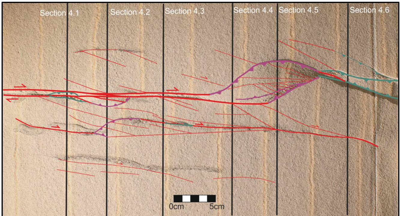
Fig. 87. Top View of the model after the end of the strike-slip phase. A transparent view of fig. 5 is laid over the end of the strike-slip phase. Showing that the main strike-slip faults are located above the silicon putty walls and that the pop-up and pull-apart structures are formed due to lateral variations in the distribution of the silicon putty walls.
