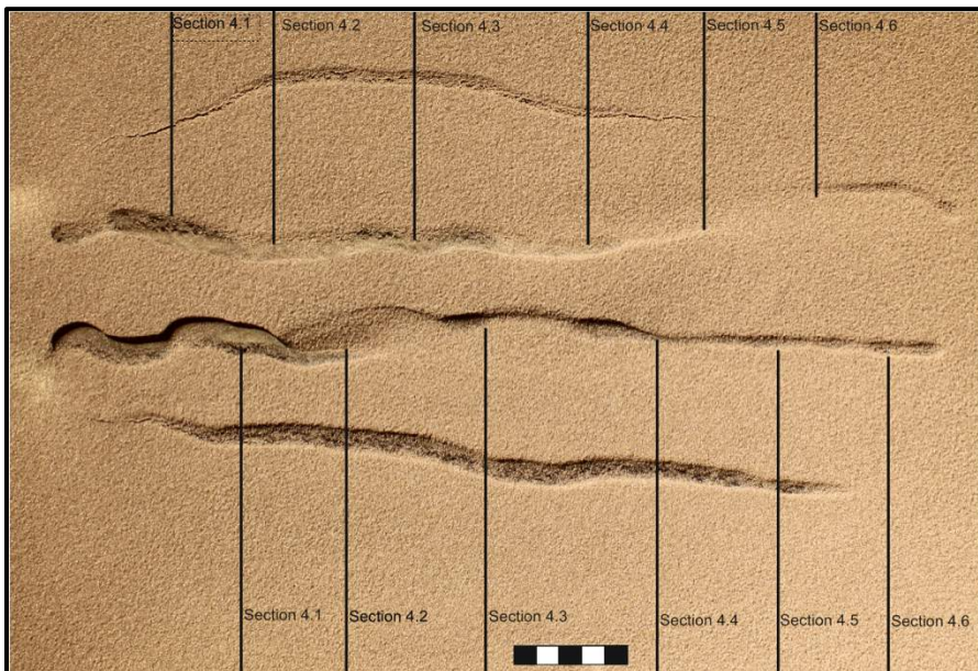
Fig. 73. Top view of model 4 after two hours of resting. The Blue part of the basin (part C) is normally filled, the white part of the basin (Part D) is underfilled with a topography difference of 5mm between the basin floor and the surrounding platforms. During this phase of the experiment, the silicon putty in the underfilled part of the basin slowly spreads towards the center of the basin by gravitational spreading.
