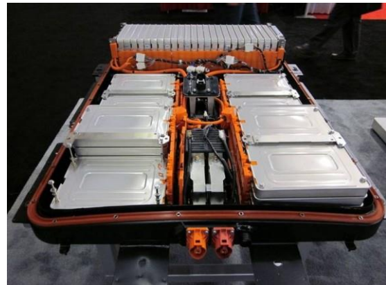
Figure 7: Nissan Leaf Pouch cell battery pack (25kWh). (Cleantechnica, 2016)
