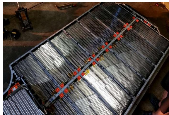
Figure 5: Cylindrical cell battery pack Tesla Model S 85. (Tesla Motors Club, 2014)
