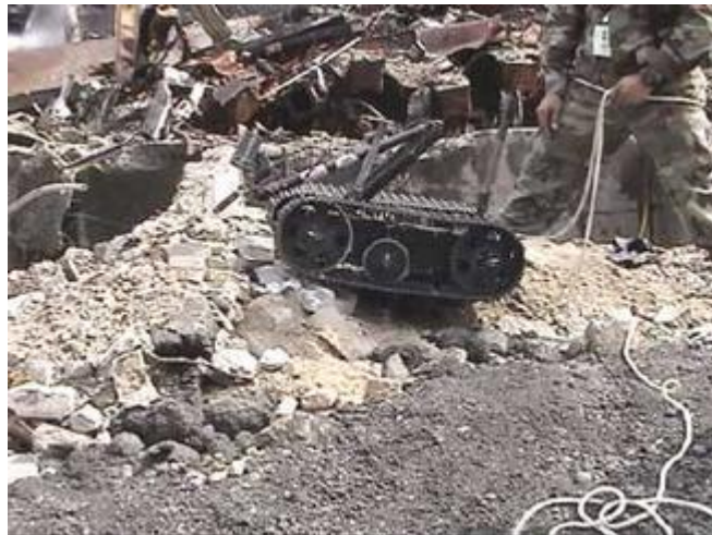
Figure 1.1. The Foster Miller Solem robot in operation 9/11. Source: fireengineering.com
