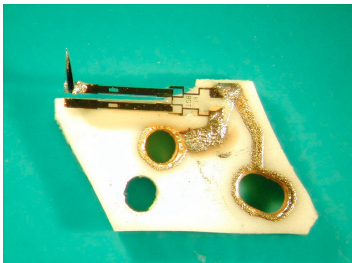
Figure 2.3: An example of a qPlus sensor. Note that one of the two prongs of the tuning fork is fixed to the white block. Image taken from ref. [24].
