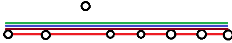
Fig. 3.4: This is an illustration of errors that can arise from the correlation between track parameters and offsets. The circles represent hits on chips. In blue the result of the Biassed simple algorithm. The red line is the line found by excluding the third chip. The green line an example of excluding say the fourth chip. The dark red line is the final result of the HIP algorithm.
