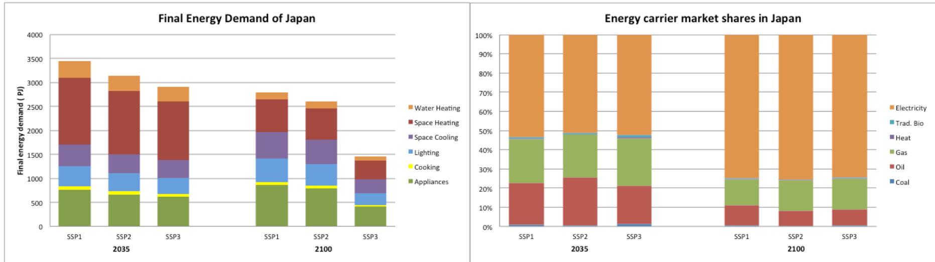
Figure 3.16&17 Final energy demand disaggregated by end-uses and energy carrier market shares of Japan. Model results for each SSP in the years 2035 and 2100.
