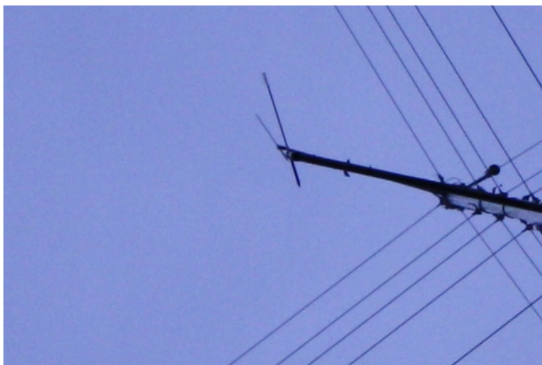
Figure 2.10: Wind veer. The foto is taken underneath the meteorological mast at the Princess Alexia site. The wind vanes are positioned at 46 and 96 meter above ground level.
