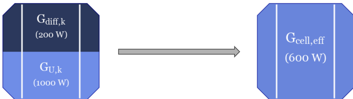
Figure 2.3c: Principle of deriving the effective cell irradiance from its shaded and unshaded fractions. In this example, \sigma_P = 50\% . Modified from previous similar work (Sinapis, et al., in press; Tzikas, 2015).
