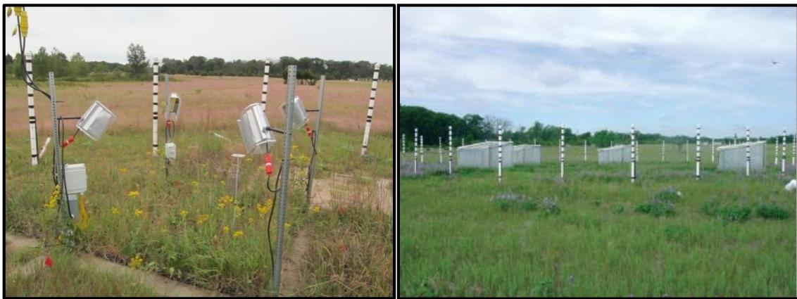
Figure 1: (Left) Photograph showing the technology for the warming treatment in a plot in the TeRaCON experiment. Photo credit: Dr. Roy Rich. (Right) Photograph showing one FACE ring and four of the portable rainout shelters used for the reduced precipitation treatment in the TeRaCON experiment. Photo credit: Kary Worm (Eisenhauer et al., 2012).
