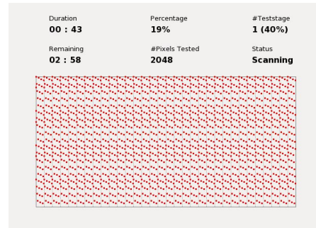
Figure 5.12: Part of the threshold scan tab which gives feedback about the progress of the current threshold scan.
