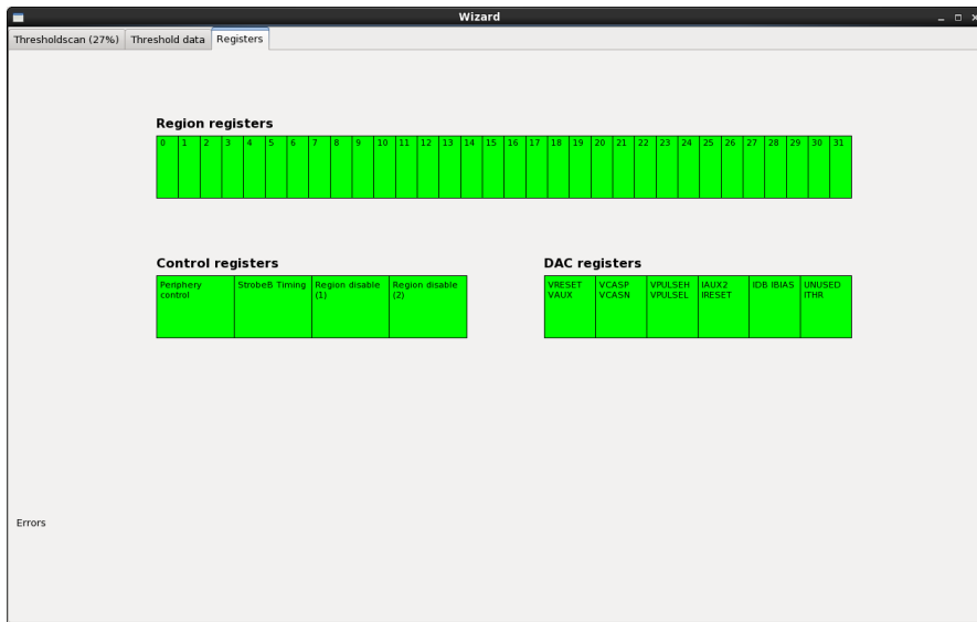
Figure 5.15: A screenshot of the register tab. It shows all tested registers. A register is shown in green if it passed the test, it turns red otherwise.
