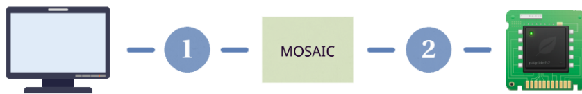
Figure 5.1: A schematic overview of the measuring set used by the software. The computer is connected to the MOSAIC board by an ethernet gigabit cable (1). The MOSAIC board on his turn is connected to the chip with a custom made cable (2).
