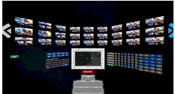
Fig. 1. An overview of the VR lifelog retrieval system, with the Map located in the center, with the DateTime and Tag interfaces on the right and left respectively. In the top half, the ImageView can be seen. The select/blacklist button is located underneath the Map , with two displays containing the number of filtered images and Introduction/Retrieval queries used in the experiment.
