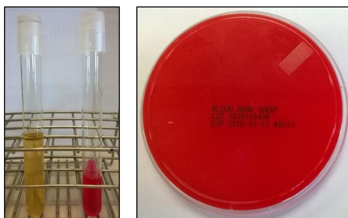
Figure 14 Some of the materials used for the confirmation of presumptive Listeria monocytogenes colonies. (From left to right: tryptone soya yeast extract broth (TSYEB), phenol red broth, and a sheep blood agar plate.)
