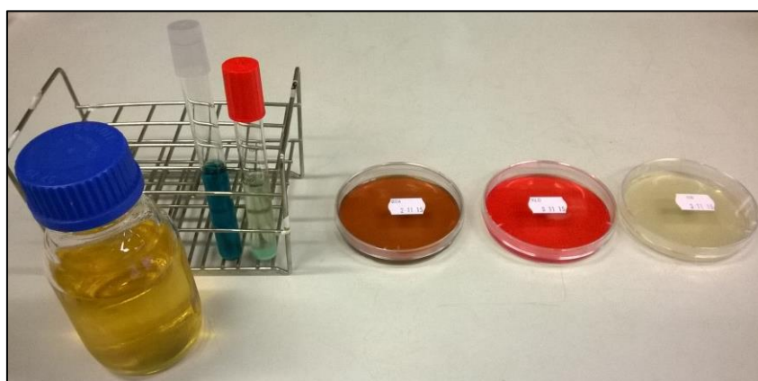
Figure 21 Materials used for the detection and enumeration of Salmonella species. (From left to right: buffered peptone water (BPW), Rappaport Vassiliadis (RV) broth, Muller-Kauffmann tetrathionate-novobiocin (MKTn) broth, brilliant green agar (BGA), xylose lysine deoxycholate (XLD) agar, and nutrient agar (NA).)
