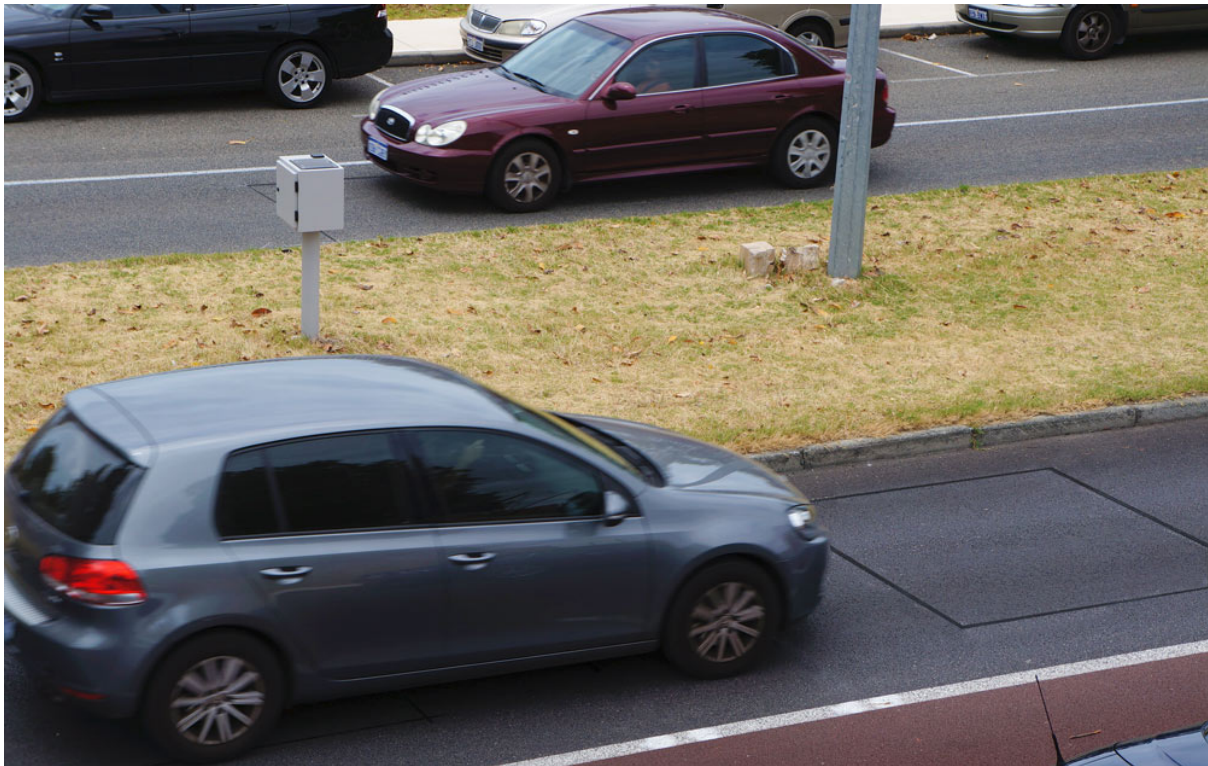
FIGURE 5.12: This inductive loop detector system is ubiquitous in the Dutch road network. The vehicle counts obtained through this system can be used to evaluate the travelling population inferred from the mobile phone location data.
