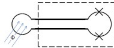
Figure 2.1 Schematic representation of the SQUID sensor extended with a circular pick up loop. The dashes area is magnetically shielded. [Reith, 2015]
