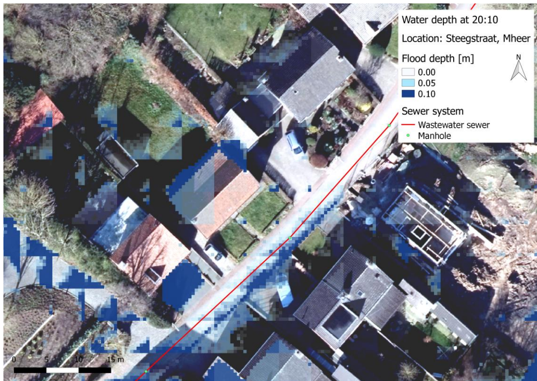
Figure E-7: Flood map of the Steegstraat flood location after simulation of the rainfall event of 18 August 2011.
