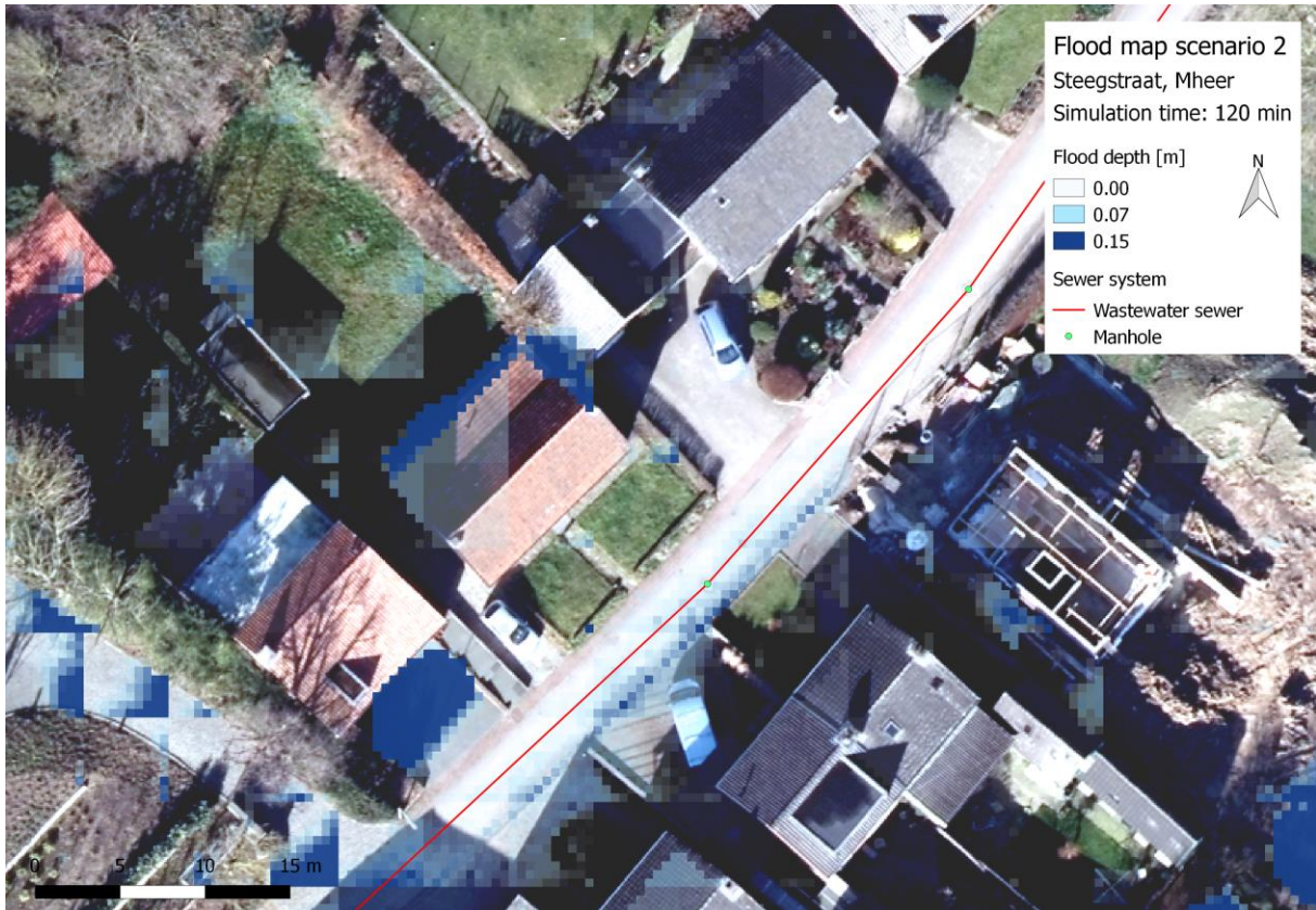
Figure 4-11: Flood map at the Steegstraat after 2 hours of model simulation during rainfall scenario 2.
