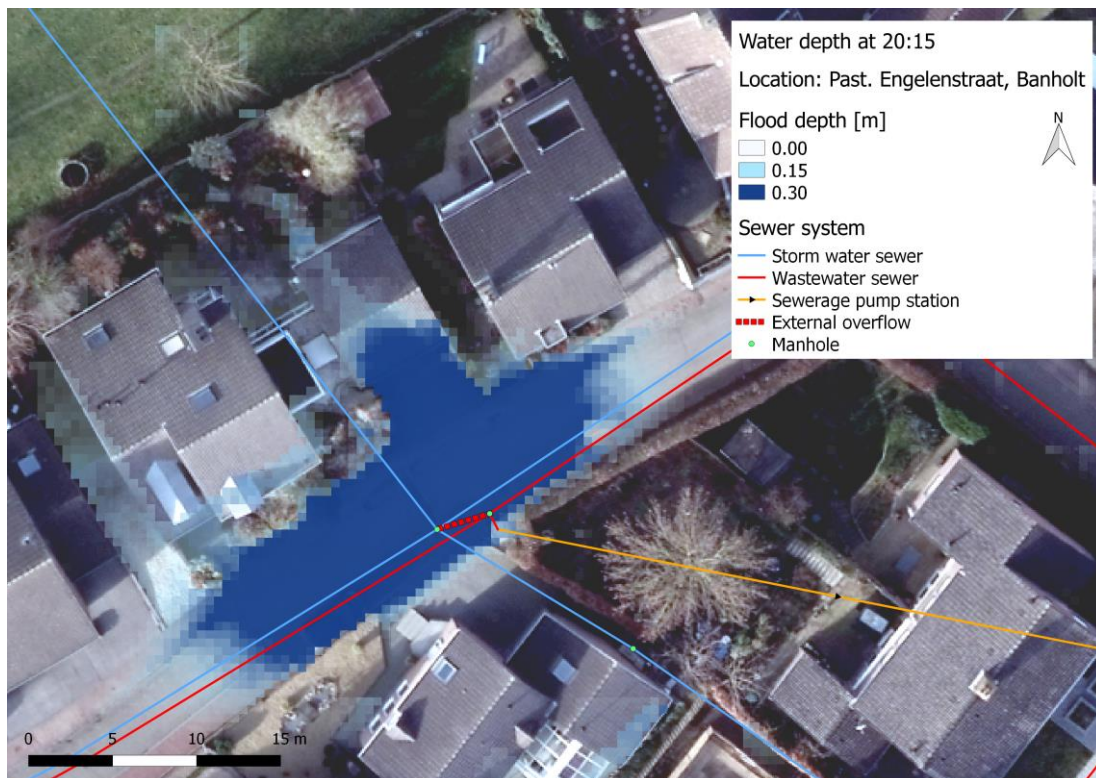
Figure E-11: Flood map of the Pastoor Engelenstraat after simulation of the rainfall event of 18 August 2011.
