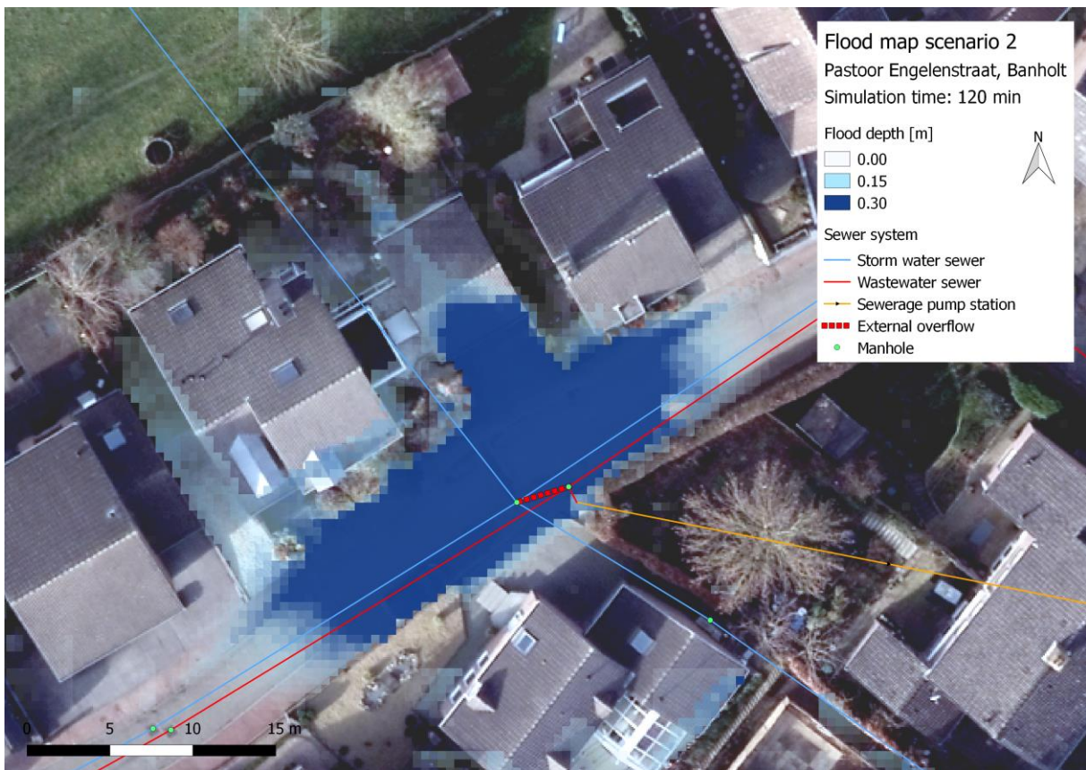
Figure 4-24: Flood map at the Pastoor Engelenstraat after 2 hours of model simulation during scenario 2.
