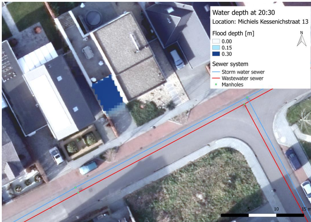
Figure E-17: Flood map at the Michiels Kessenichstraat 13, Mheer shows flooding at the sloping driveway.
