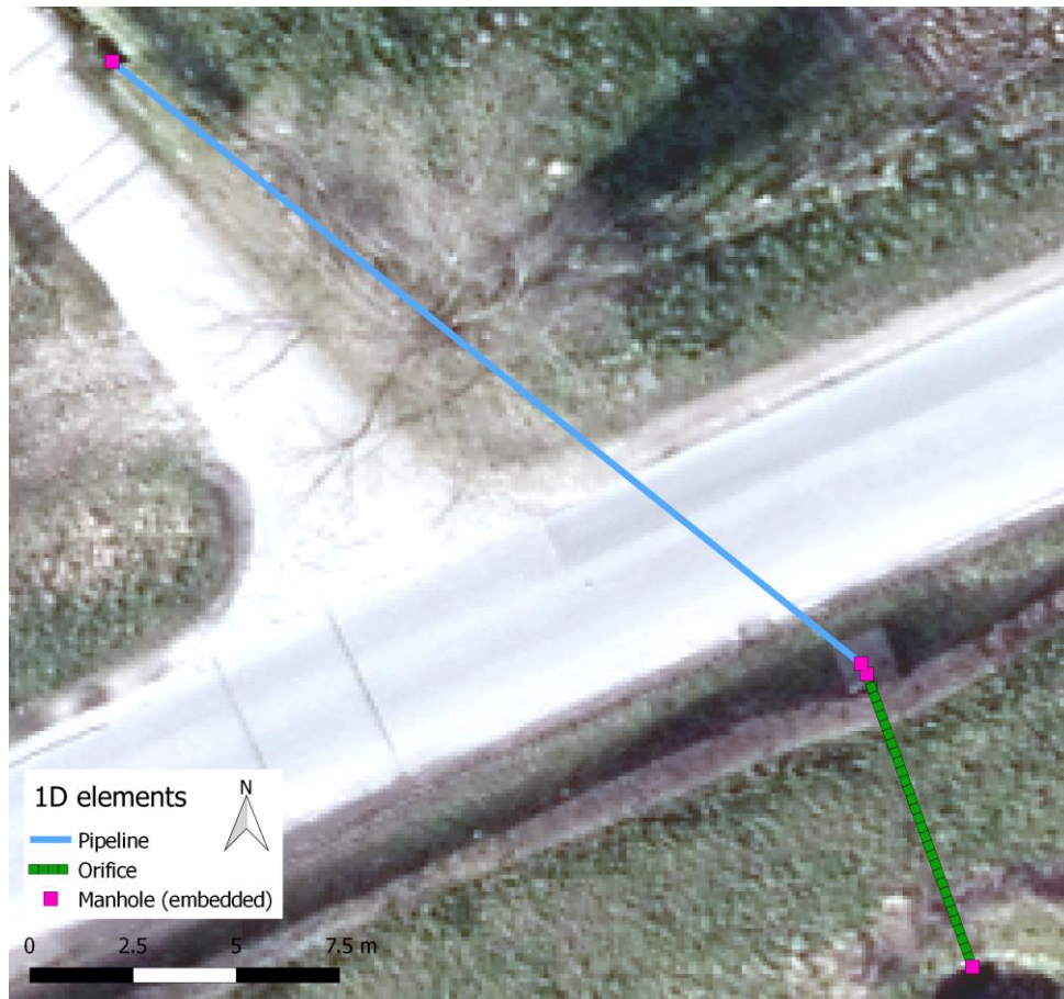
Figure C-1: Schematization of a culvert and outlet of a water storage buffer in 3Di.
