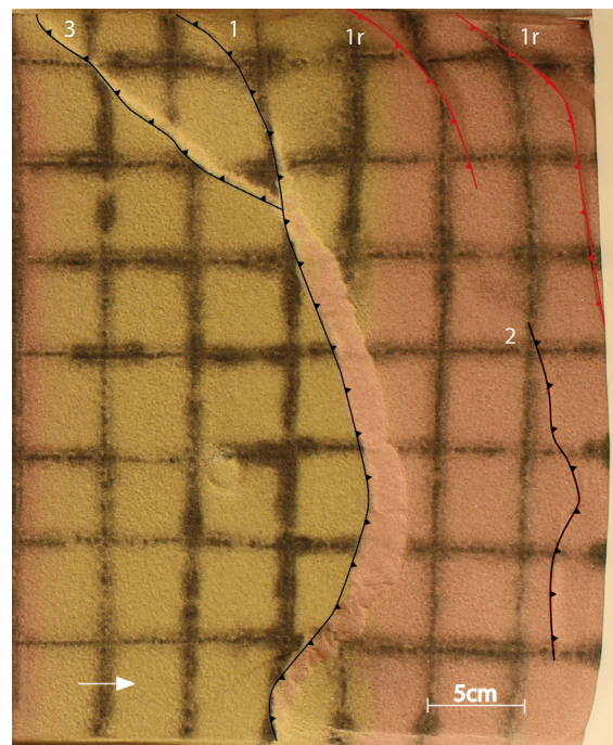
Fig. 51. Fault distribution observed on the surface of model 4 after 5% of BS.
