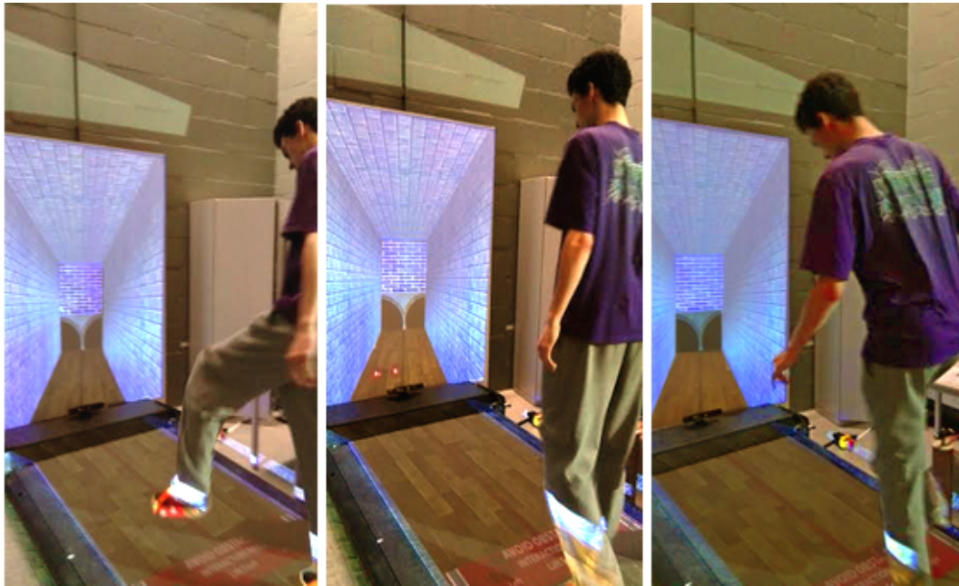
FIGURE 2.6: Different behaviors that the subjects have to perform while Walking on the treadmill, with constant speed. The subjects have to lift their right or left foot respectively. to step over virtual obstacles appearing in their path.
