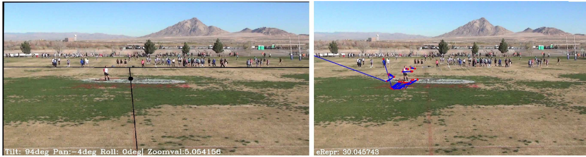
Figure 5.5: Initial camera parameters. On the left is the outcome from the player point correspondences, and on the right is the outcome from manual optimisation.
