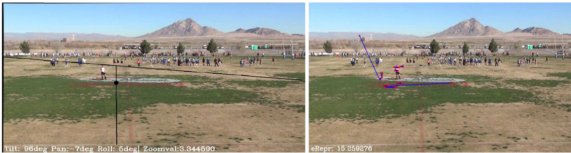
Figure 5.4: Initial camera parameters. On the left is the projection of the field onto the image plane. On the right, the projected GPS points are connected to the hand-picked player locations. The camera parameters were found by iteratively solving the PnP problem using a Levenberg-Marquardt optimisation.
