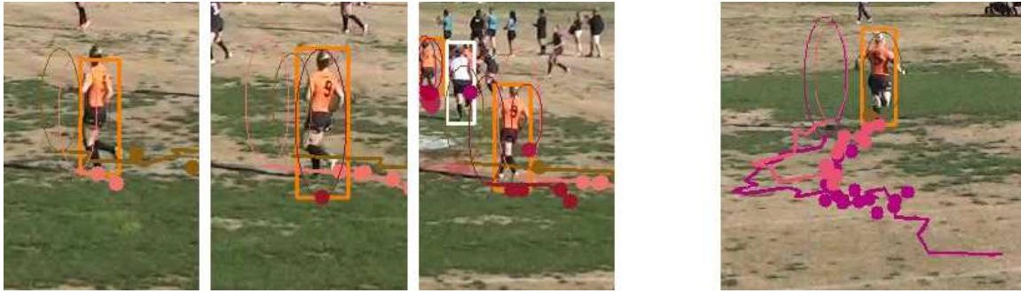
Figure 5.16: Consecutive detections being assigned to two overlapping tracklets. On the left, the progress is shown in three frames. On the right an example is given, where the ground plane path history of the tracklets show a similar situation.
