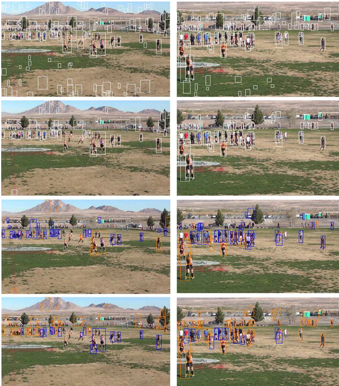
Figure 5.13: Visualisation of player detection results for the different filters. For both frames, the detector confidence level was set at -1.3. From top to bottom: player detector, background removal, assignment using all histograms (threshold=5), and on the bottom the selective colour descriptor (threshold 8.5).
