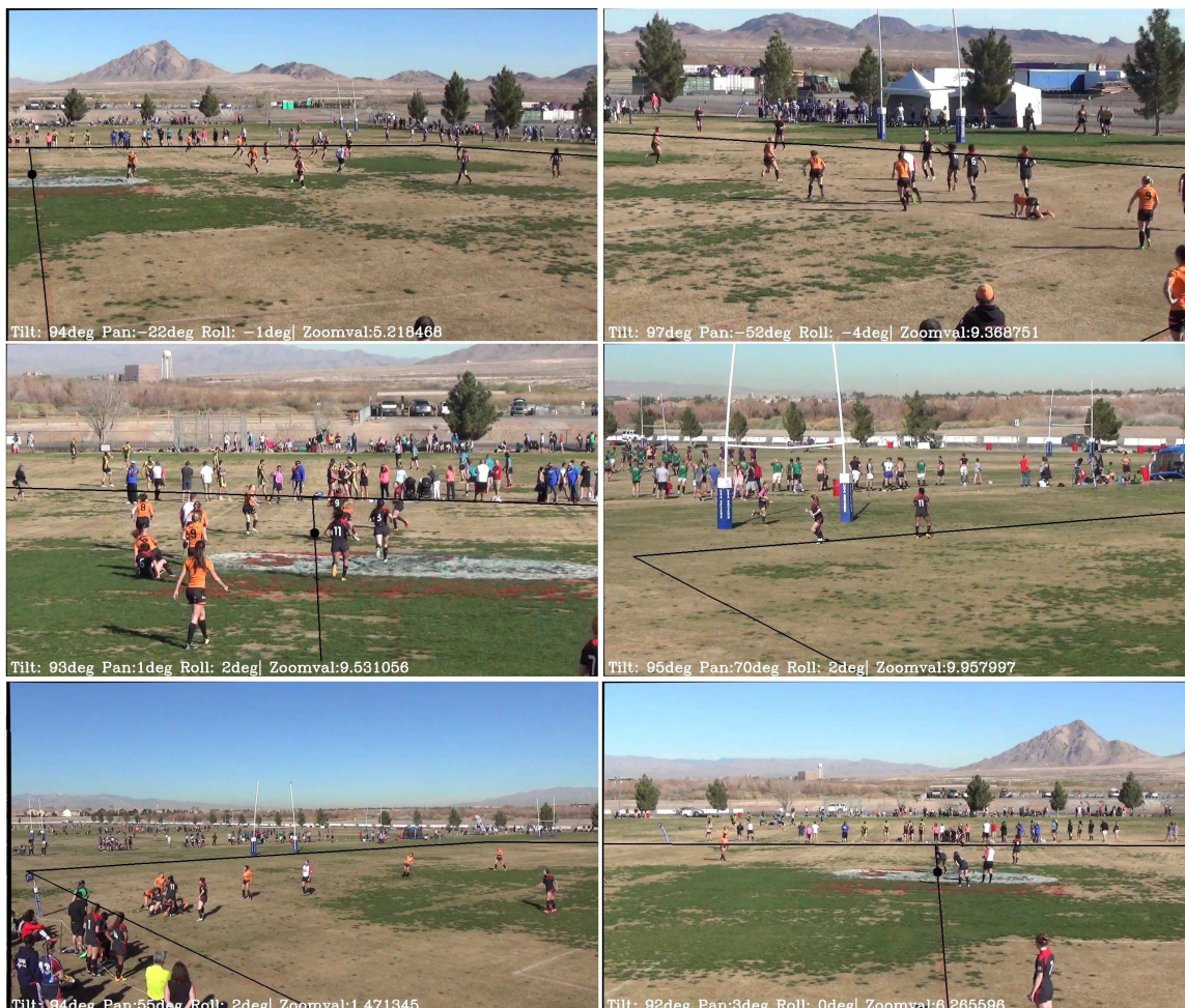
Figure 5.6: An image sequence portraying the projection of the field lines onto them. It shows several successful and unsuccessful projections.
