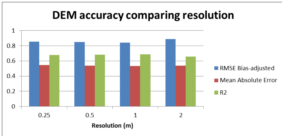
Figure 33: Accuracy of the available grid sizes compared. RMSE and MAE, closer to 0 is better. R^2 is coefficient of determination, closer to 1 is better.
