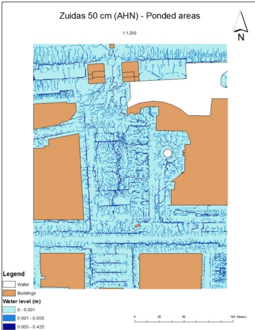
Figure 49: Example ponded area (at least 0.005 m) (between 0.001-0.005 m) in the Zuidas area for the AHN DEM
