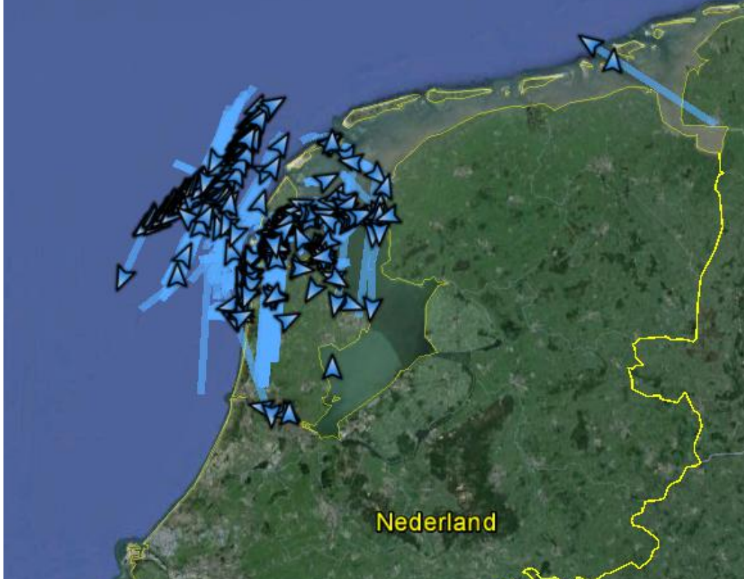
Figure 5.3: All vessel tracks received on 09-09-2014 by a single antenna, plotted with Google Earth. (Tracks over land typically correspond to a ship of which in-between data was absent.)
