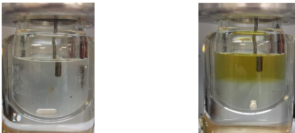
Figure 1 - Previous TNO experiments showing the unloaded (L) and loaded (R) blend. The loaded blend clearly shows that two distinct phases have been formed, as can be seen from the colour difference.
