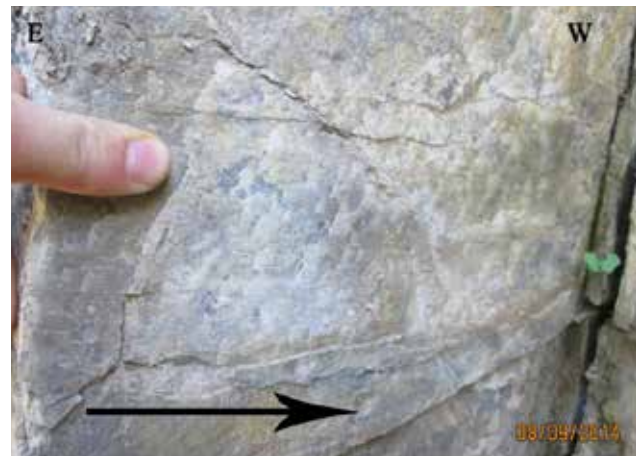
1.3b. Slickenside with steps indicating dextral shear.
