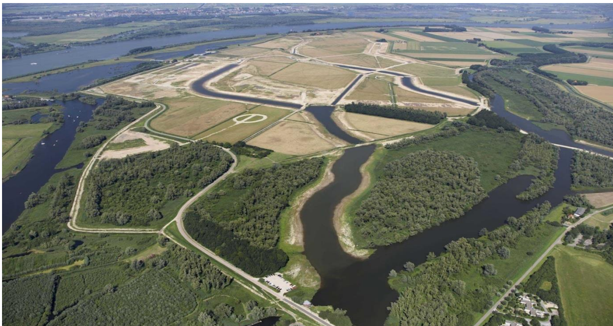
Figure 3.4: Overview of 'De Kleine Noordwaard', showing the channels dug into the former polder area. (Source: bvkoek.nl)
