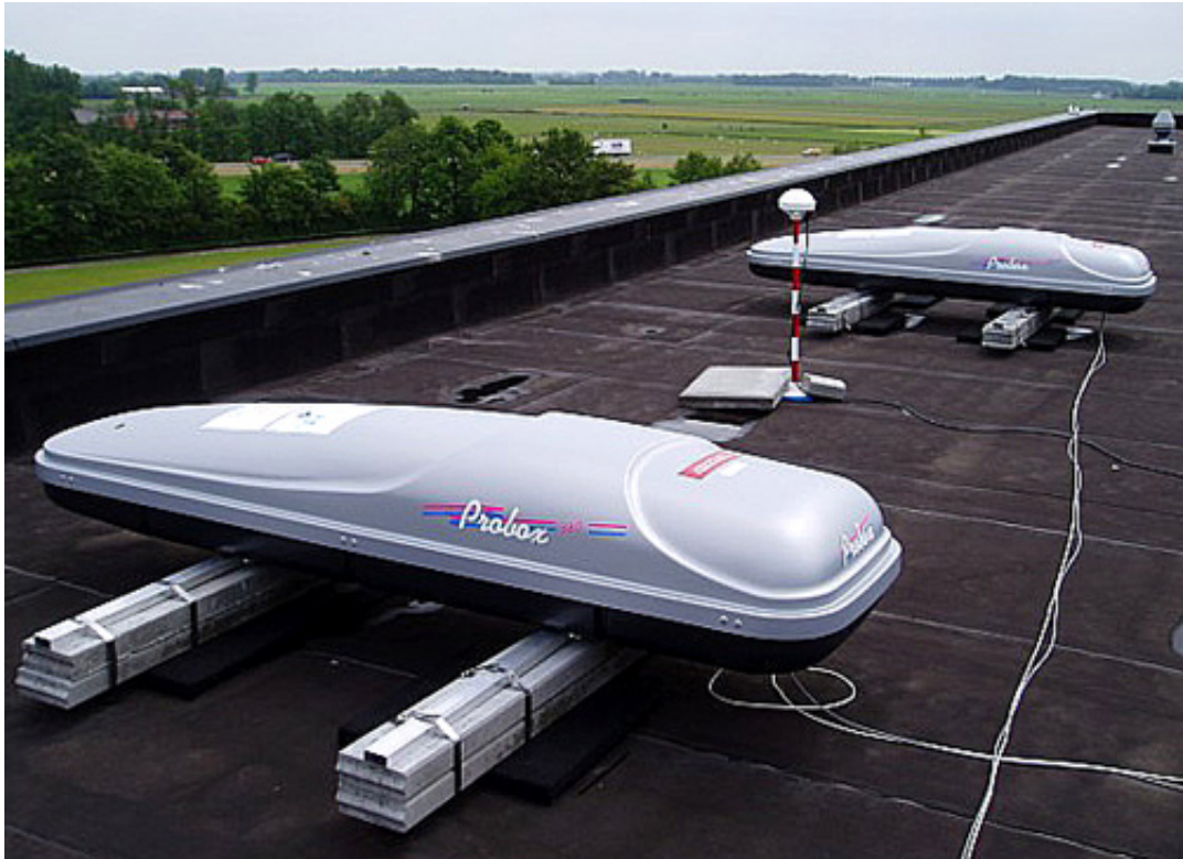
Figure 3.2: Example of HiSparc detector setup on the roof of a high school. Source: http://www.ru.nl/publish/pages/542007/skiboxen-op-dak-school.jpg
