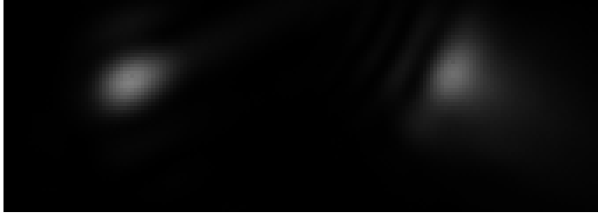
Figure 3.2: A camera image. On the right it shows the reference beam. On the left the focus can be seen.
