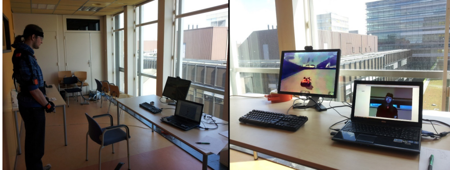
Figure 6: Left: The entire setup, with a racing user. Right: (edited for clarity) The left screen shows the game, at which the user is looking, the right screen shows the tracker and how it is currently tracking the user.
