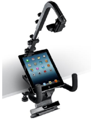
Figure 2. The eye-tracker is placed on the stand base, and the iPad is attached in the centre. Adopted from Shayan, Abrahamson, Bakker, Duijzer and Van der Schaaf (2014).
