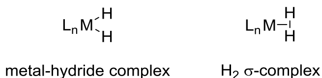
Figure 5: Structural representation of the metal-hydride and \sigma -bound hydrogen complexes.
