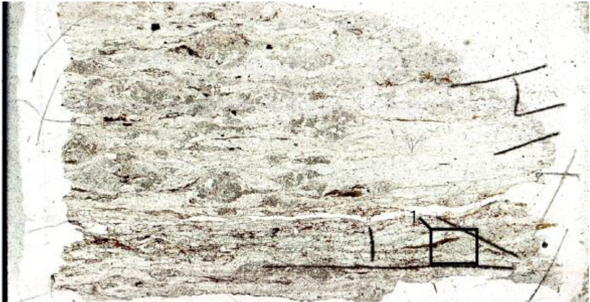
Figure 11 - Thin section scan of sample 14. Rectangle labeled 1 represents the more specific, smaller area analyzed with the OM, of which (Leica) images made, are presented in the report and the appendix 2.2 (Optical Microscopy). The arrow located on the bottom of the thin section indicates plunge of the sample. The small, vertical line positioned on the arrow indicates the direction of the top of the sample.
