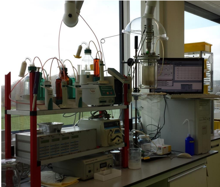
Figure 4.2.2. The experimental setup with the bioreactor for open CO 2 system experiments.
