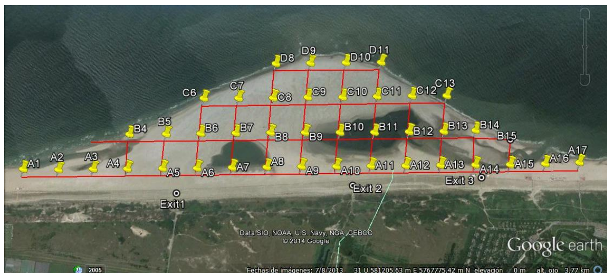
Figure 3. The distinct shape of the mega nourishment the Sand Motor. The sampling grid of 250 x 250m that was used for the results described in appendix C and the fieldwork in this research (section 4.1).
