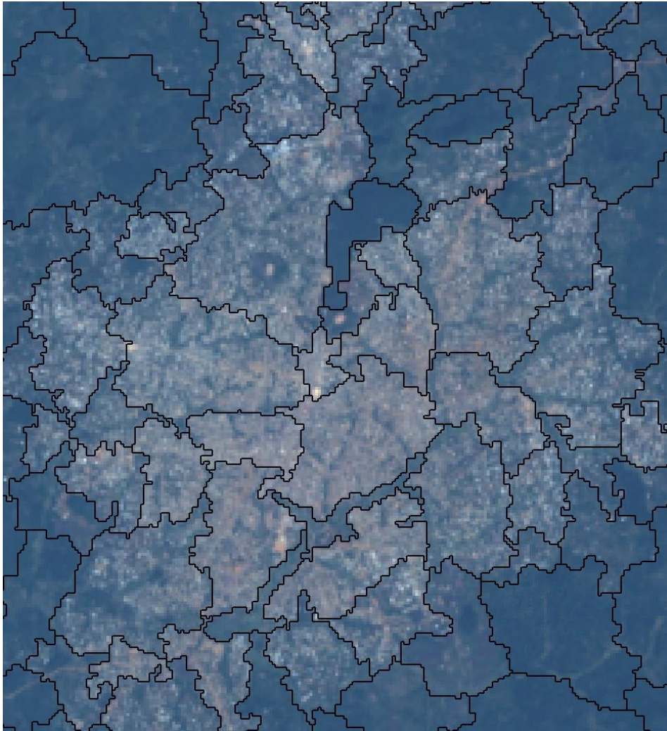
Figure 46. Segmentation of the main urban area of transect 1 – 2013 (true colour) using the parameter values from Maxwell (2010): shape = 0.1, compactness = 0.9 and scale = 20.
