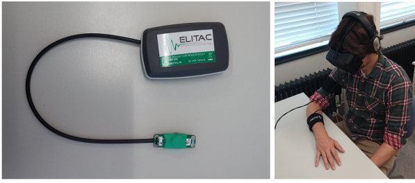
Figure 1: The measurement setup; (left) the Elitac control module and a single factor, (right) a participant sitting in the correct position wearing the HMD, tactile sleeve and headphones.
