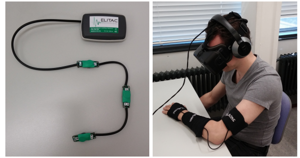
Figure 6: The measurement setup; (left) the Elitac control module and three tactors, (right) a participant sitting in the correct position wearing the HMD, wireless headphones and tactile sleeve.
