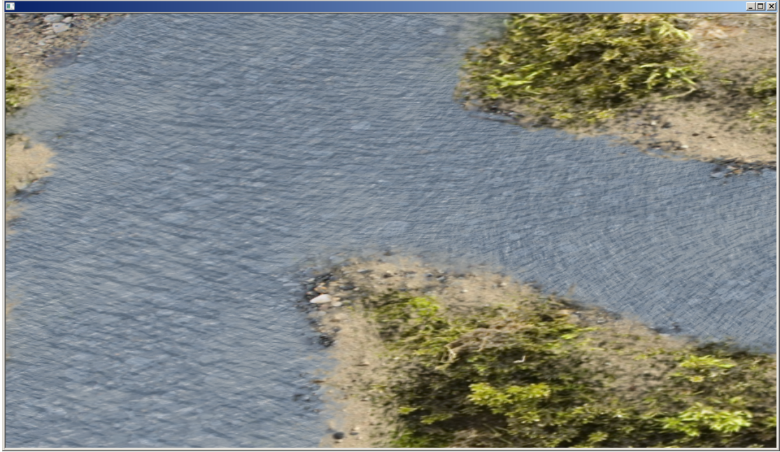
Figure A.3.: Tiled directional flow with animated normal maps, generated with the FFT.
