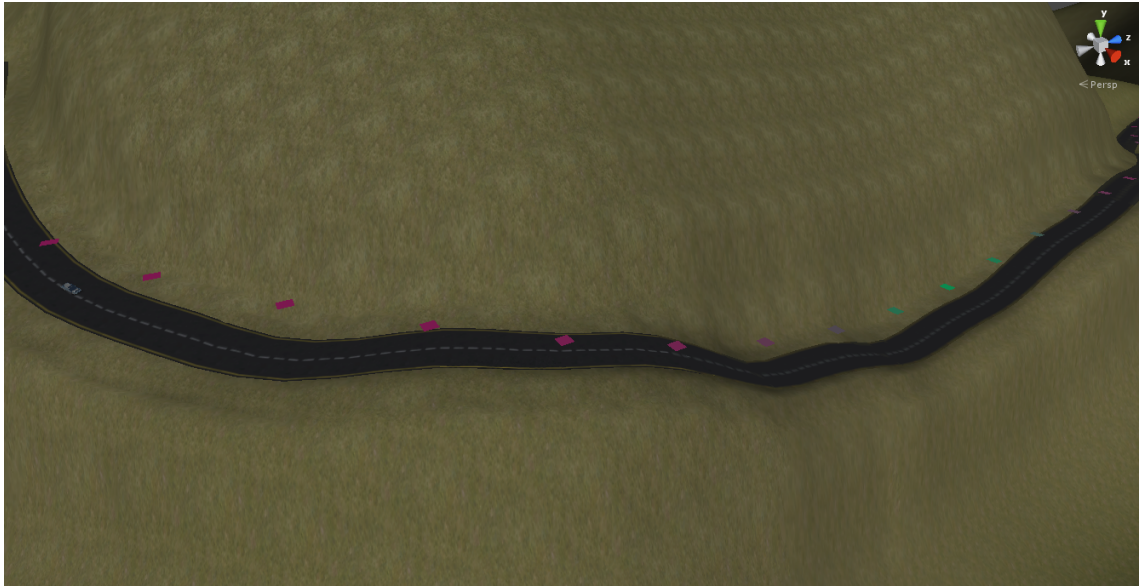
Figure 5.2: Markers floating above the road visualize the calculated maximum safe velocity v , ranging from high (green) to low (red).
