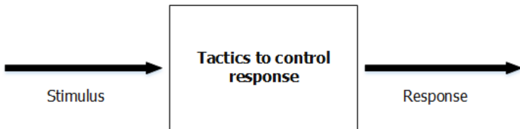
Figure 13 - The role of tactics to influence and control the response to a certain stimuli (Bass et al., 2012)
