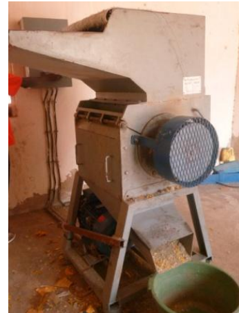
Picture 12 : Crushing machine transforming large plastic pieces into chips (in the valorization center of Kaolack)
