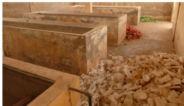
Picture 9 : Baths where plastic pieces are manually washed (valorization center of Kaolack)
