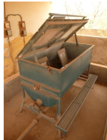
Picture 13 : Washing machine for plastic pieces (in the valorization center of Kaolack)
