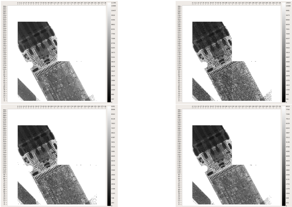
Figure 9: A USB memory stick at a threshold of 50 ADCU (top-left), 60 ADCU (top-right), 70 ADCU (bottom-left), and 80 ADCU (bottom-right).
